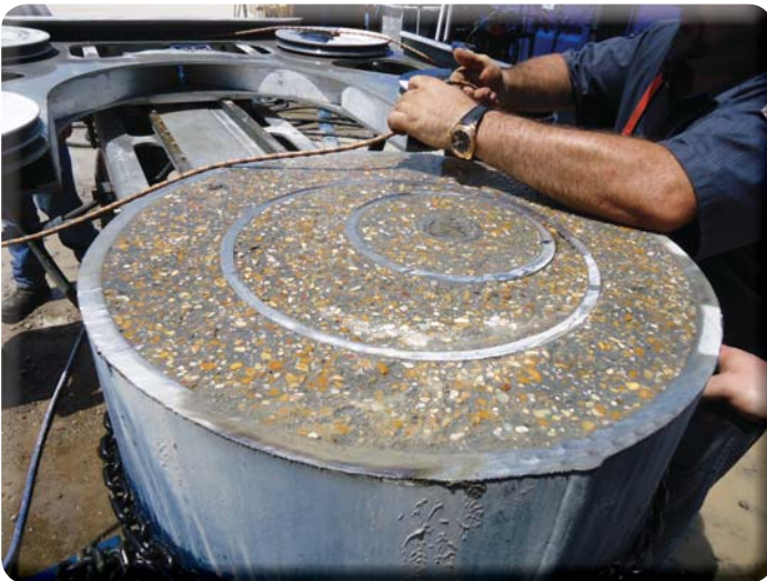
Multi-String Cut made with Mactech's DWS-26i Diamond Wire Saw
